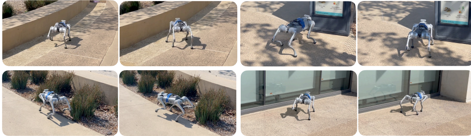
Figure 11: Obstacle avoidance screenshots. Locomotion policy can ensure collision-free in the face of high grass, certain transparent glass, and large objects under strong sunlight. The policy presents robustness on sand and grass terrains.
