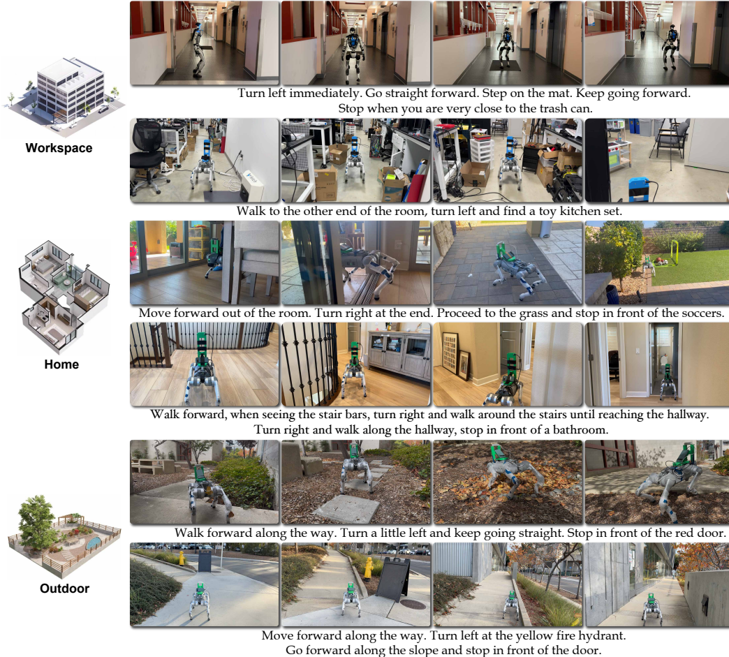
Figure 1: Real-world demonstration of NaVILA: Upon receiving human instructions, NaVILA uses a vision-language model to process RGB video frames and employs locomotion skills to execute the task on a robot. The robot successfully handles long-horizon navigation tasks and operates safely in challenging environments.
